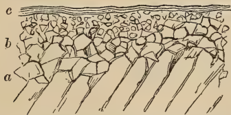
FIG. 92.—SECTION SHOWING THE UPWARD PASSAGE OF ROCK (a) INTO SUBSOIL (b) AND THENCE INTO VEGETABLE SOIL (c).
